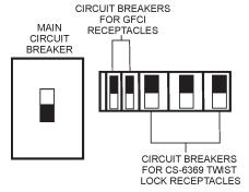
Figure 42. Main, Aux. and GFCI Circuit Breakers (OFF)
